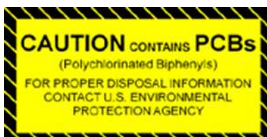
FIGURE 2: Small PCB MarkLabel, shown actual size (1 inch by 2 inches)
