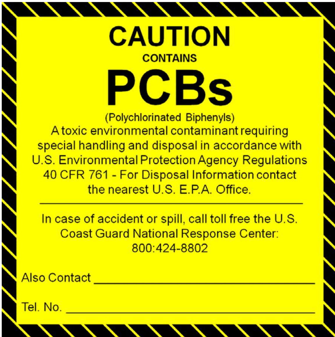
FIGURE 1: Large PCB Mark/Label, shown actual size (6 inches by 6 inches)
